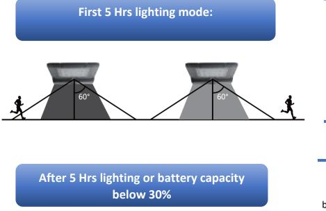
Automatically turns on to full brightness when motion is detected in the range ≤ 8mtrs and then turns to weak, brightness in 20 seconds of no motion.
