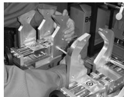
Fig. 3 Montarea bacurilor de prindere prismatice Mount the prism clamping jaws
